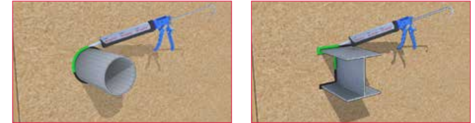
Fig.4: Sealing gaps and cracks with Wraptite Liquid Flashing. Refer to Wraptite®: Membrane & Accessories Installation Guide for full details.
