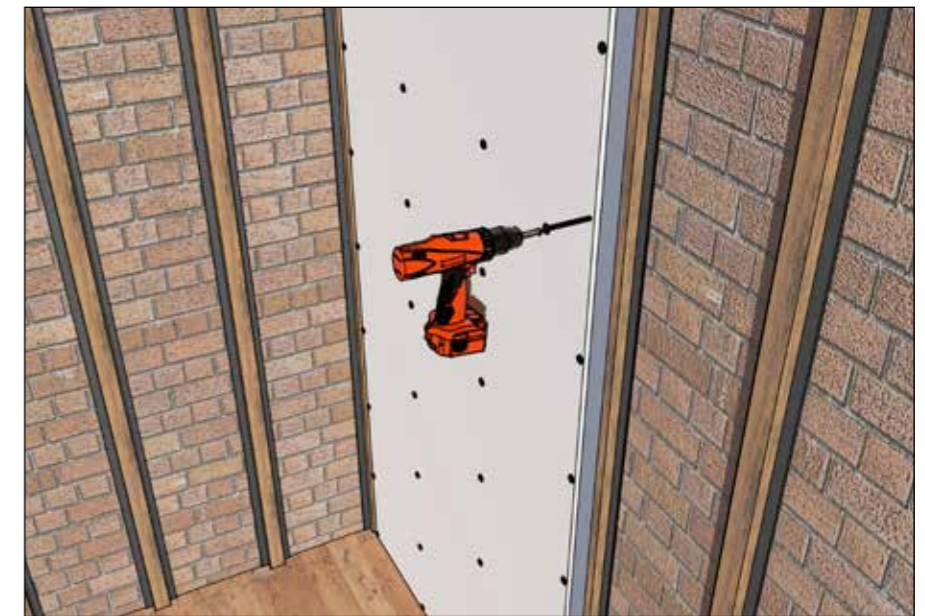
Fig. 4 Fixing Spacetherm Wallboard to timber straps
