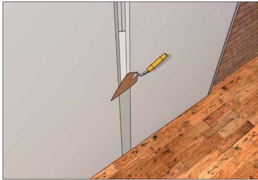
Fig. 8 Taping and Filling Joints in Spacetherm Wallboard
