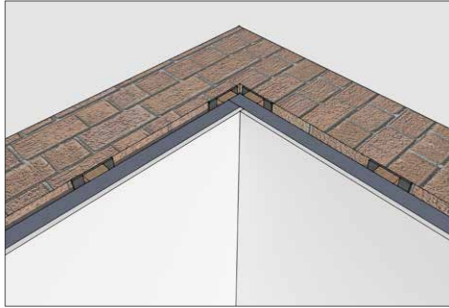
Fig. 6 Internal Angle Joint in Spacetherm Wallboard / Spacetherm A2 Wallboard
