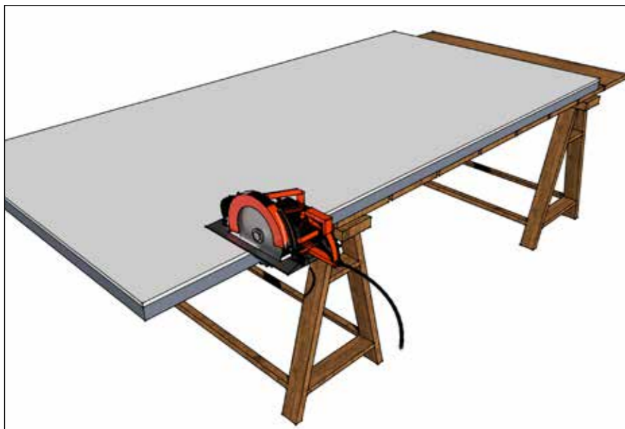
Fig. 2 Cutting Spacetherm Wallboard / Spacetherm A2 Wallboard boards
