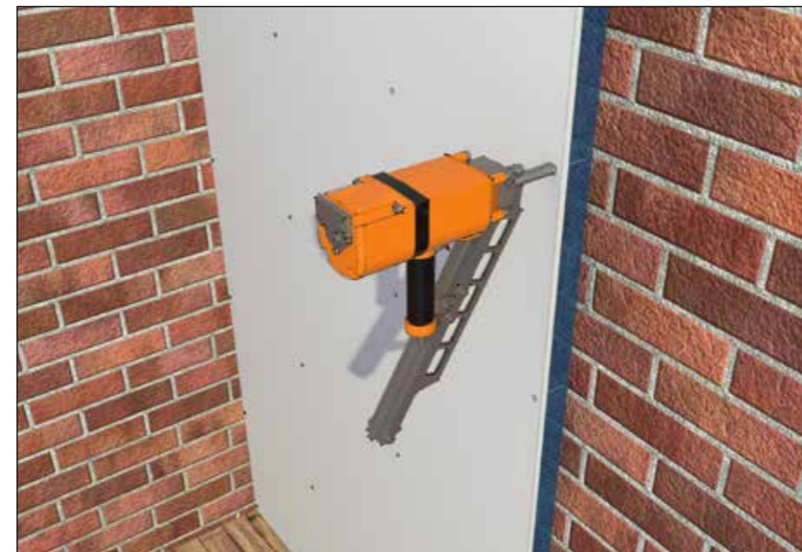
Fig. 4 Direct fixing Spacetherm Multi using nailgun
