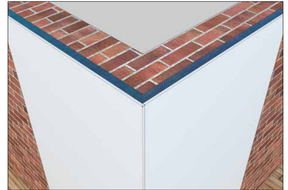
Fig. 5 External Angle Joint in Spacetherm Multi
