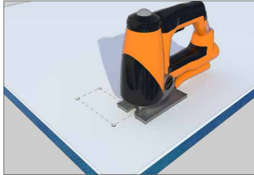
Fig. 3 Making cut-outs in Spacetherm Multi / Spacetherm A2 Multi
