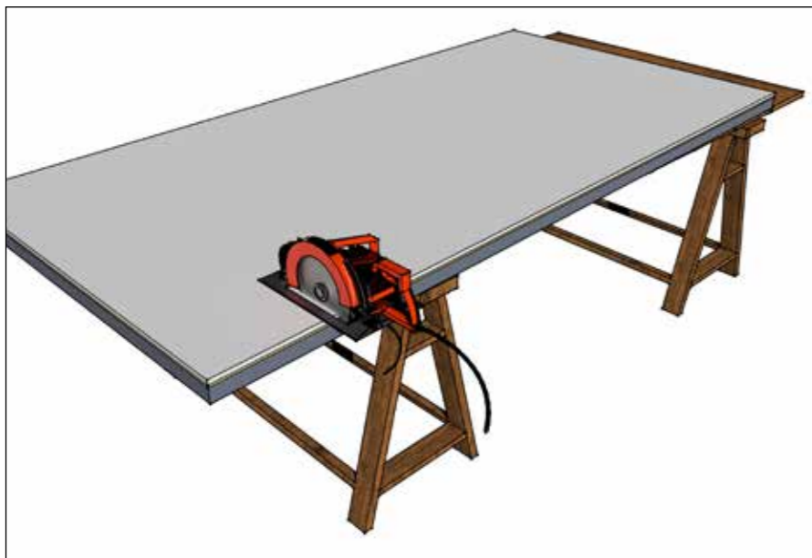
Fig. 2 Cutting Spacetherm Directfix / Spacetherm A2 Directfix Boards
