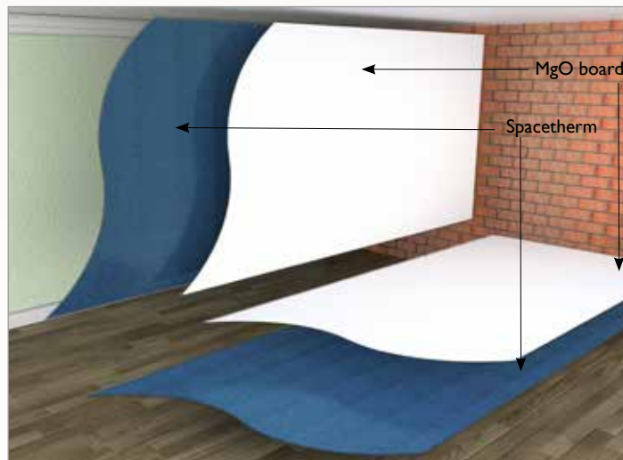
Image showing Spacetherm Multi applied internally to an existing external wall structure.
