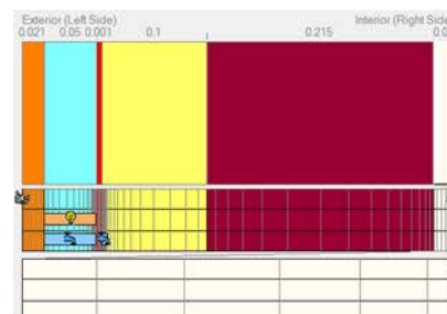
Rainscreen Brick Wall with external PIR/Rockwool
